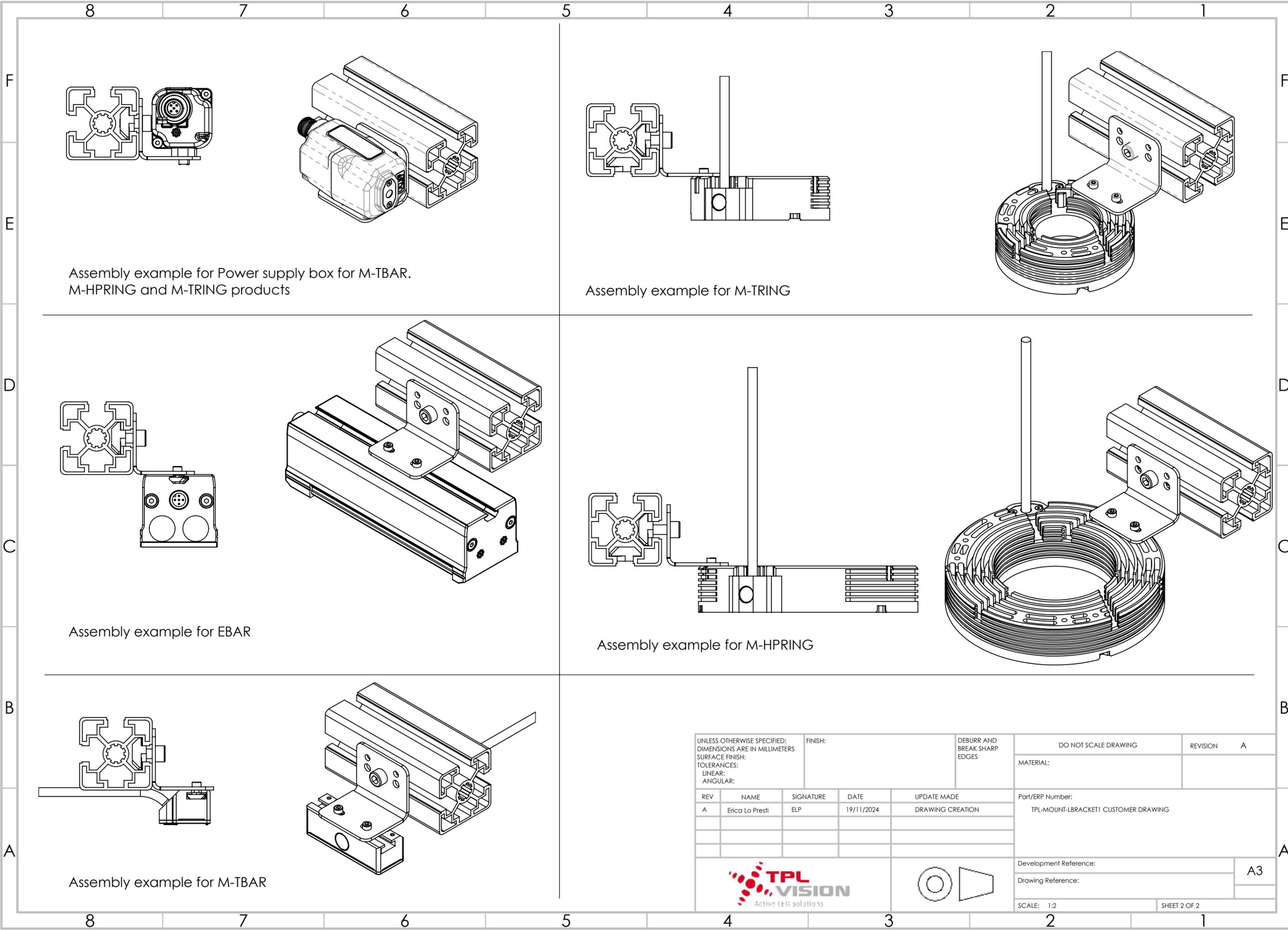
Assembly example for Power supply box for M-TBAR.
